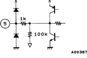
A00387 | • Grounded to $V_{REF}$ through a 1 k $\Omega$ resistor when low boost is on (pin 41: floating).                     |
