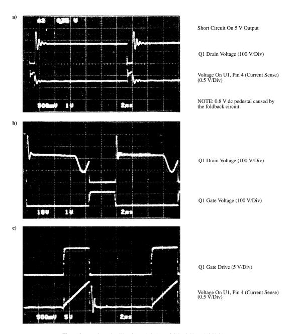
Figure 2. Operating Waveforms (all photos full load,  $V_{in} = 150 \text{ V dc}$ )
