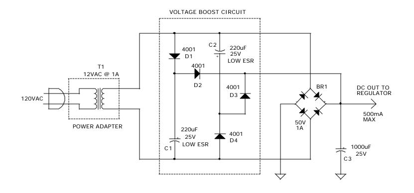
WITH 105VAC LINE VOLTAGE, 1000uF CAP ONLY, DC OUTPUT = 11.5 VDC
