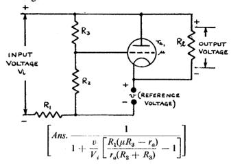
115. The equivalent circuit of a series-valve stabilizer is illustrated. Find the change in output voltage for a 10% change of input voltage if  $R_1 = 10 \text{ k}\Omega$ ,  $R_2 = 1 \text{ M}\Omega$ ,  $R_3 = 16 \text{ M}\Omega$ ,  $V_i = 2,700 \text{ V}$ , v = 100 V,  $\mu = 300$ ,  $r_a = 100 \text{ k}\Omega$  and  $R_i = 260 \text{ k}\Omega$ .
