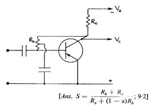
163. A transistor bias stabilization circuit is illustrated. Show that the stability factor S is given by  $(R_b + R_e)/(R_e + R_b(1 - \alpha))$  where  $R_b = R_1 R_2/(R_1 + R_2)$ .
