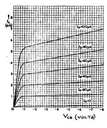
80. For a transistor used in the common-emitter configuration the relationship between collector current and collector voltage, with various fixed values of base current, are given in the following Table.
