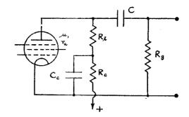
Assuming that  $R_g$  and  $r_a$  are large with respect to  $R_l$ , that the shunting effect of C and  $R_g$  on the load is negligible and that  $R_g$  is large compared with the reactance of C, show that if  $C_gR_l = CR_g$  the low-frequency gain is independent of frequency.
