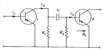
Draw an approximate high-frequency equivalent circuit for the common-base transistor arrangement and show how the high-frequency response of an RC-coupled common-emitter amplifier may be calculated.
