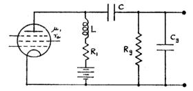
Analyse the circuit to find a desirable relation between L,  $C_{\varrho}$  and  $R_1$ . [Ans. For best flatness of the response curve  $L=0.414~C_{\varrho}R_1^2$  but a single value of L is not satisfactory for simultaneous flat gain and constant time delay and a compromise is necessary.]
