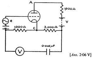
82. Draw the equivalent circuit of the arrangement shown and find the r.m.s. a.c. anode current in the valve. The valve constants are  $\mu = 20$  and  $r_a = 5,000 \Omega$ .
