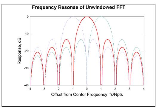
Figure 1.  $sin(N\pi f)/sin(\pi f)$  Filter Response
