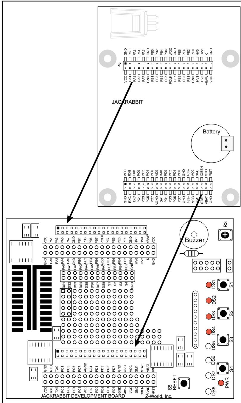
Figure 2. Attaching Jackrabbit Board to Prototyping Board
