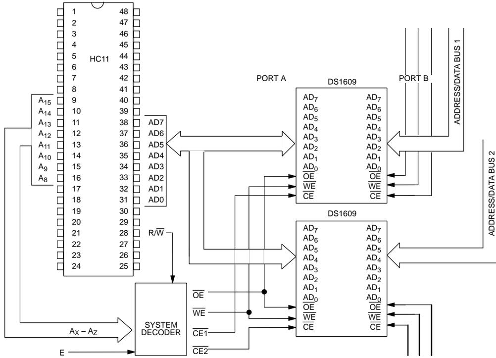
The DS1609 can be used as a go between with non-multiplexed microprocessors such as the Intel 386 or Motorola 68030. Processor cycles to and from a
