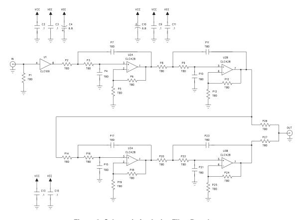
Figure 6: Schematic for Active Filter Board
