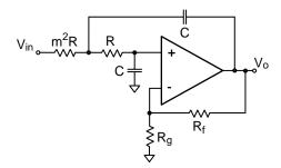
Figure 1: Sallen-Key Low Pass Filter with Equal Cs
