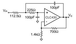
Figure 2: Example of Low Pass Filter
