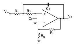
Figure 5: Low Pass Sallen-Key Filter
