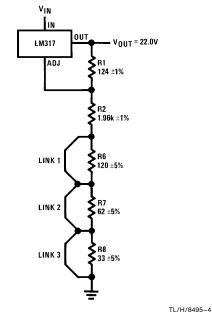
If  $V_{OUT}$  is lower than 20.90V, snip link 1 (if not, don't). *Then* if  $V_{OUT}$  is lower than 21.55V, snip link 2 (if not, don't). *Then* if  $V_{OUT}$  is lower than 21.82V, snip link 3 (if not, don't).
