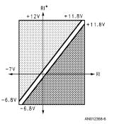
FIGURE 6. Receiver Input Range
