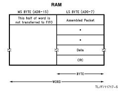
FIGURE 4. Packet Assembly for Loopback Work Wide Transfers
