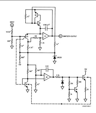
\*1% metal film resistor †Polystyrene Q2 = 2N2222A Q5 = 2N2907A A1, A2 = LF412 dual Q1, Q3, Q4, Q6 = LM3046 array
