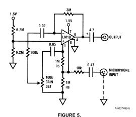
Potentially, using the reference as a preamplifier in this fashion can cause excess noise. However, because the reference voltage is low, the noise contribution which adds root-mean-square, is likewise low. The input noise voltage in this connection is  $40~\text{nV}-50~\text{nV}/\sqrt{\text{Hz}}$ , approximately equal to that of the op amp.
