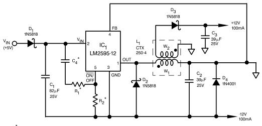
$^{\star}$  Components needed if the 5V supply is current-limited during start-up C4:  $0.1\mu F,$  ceramic
