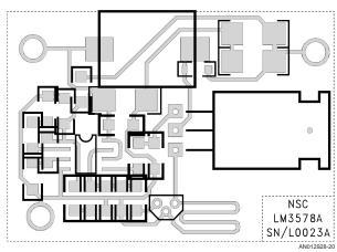
Note: Copper trace is used as current sense resistor.
