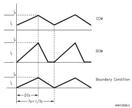
FIGURE 2. Inductor Current (i, ) Waveforms
