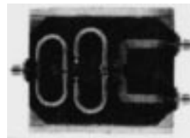
Two-section balun often used in the 100- to 400-MHz range
