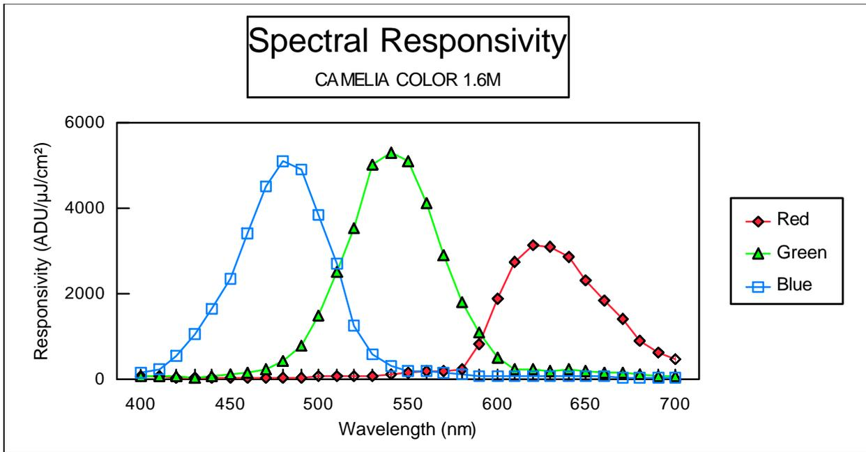
Note :  $\mu\text{J}/\text{cm}^2$  measured on the CCD chip.
