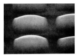
PULNiX cameras which use on-chip micro lens CCD's are called the "BL version".
