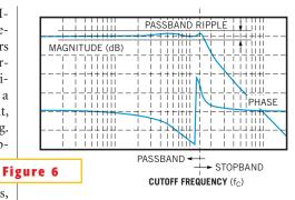
A Chebyshev filter has the best stopband characteristics but has only 3 dB of passband ripple.
