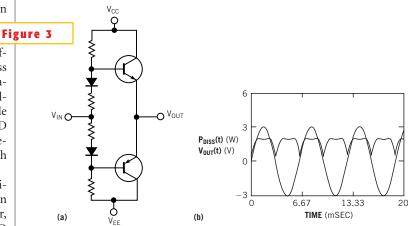
A Class AB amplifier (a) is almost as efficient as a Class B amplifier (b).
