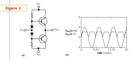
In a Class B amplifier, only one of the two series transistors in the output stage is on at a time (a). This amplifier type is more efficient than a Class A (b) but has higher distortion.
