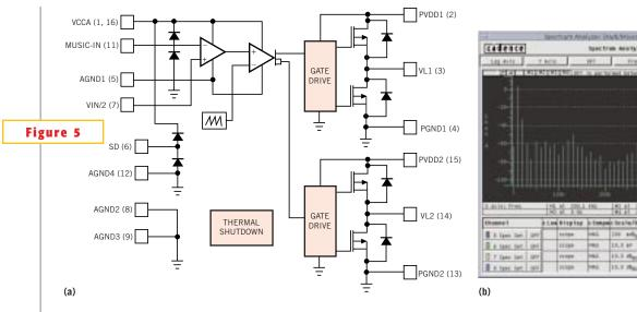
The CM8686 Class D amplifier IC uses comparators and a sawtooth generator to perform pulse-width-modulation (a). The output spectrum with an 85kHz lowpass filter shows the intermodulation products around 300 kHz (b).
