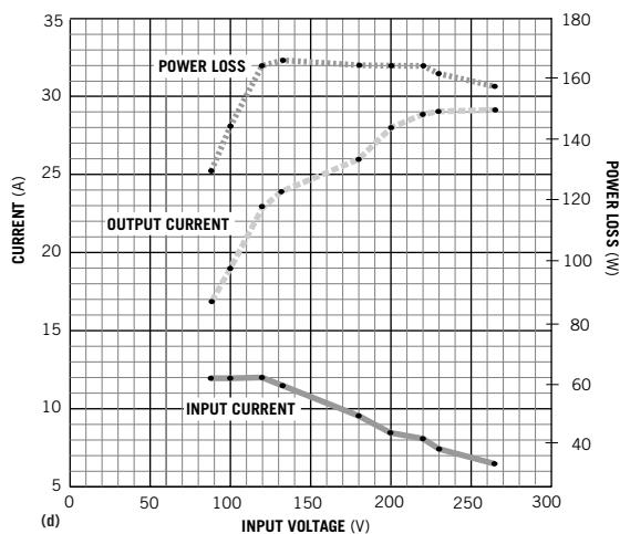
**A 48V, 23A charger with an input-current limit of 12A (a) can charge in 8.33 hours at 120V. A 48V, 23A charger with a power-loss limit of 130W (b) can charge in less than 10 hours at 120V. A 48V, 26A charger with an input-current limit of 15A at 88V (c) can charge in seven hours at 120V. A 48V, 23 to 29A charger with an input-current limit of 12A (d) can charge in 10 hours at 120V and seven hours at 230V.**
