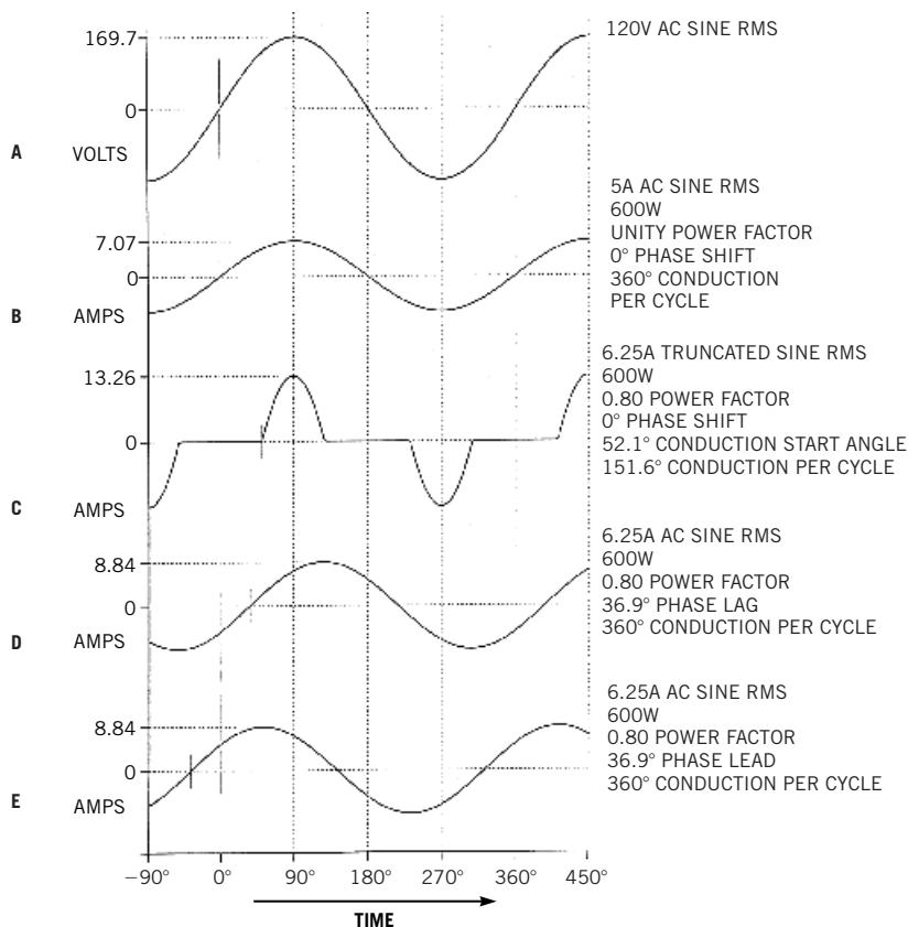
Traces A and B show the ideal relationship between voltage and current. Unfortunately, different loads cause the current waveform to stray from the ideal, as traces C, D, and E show.
