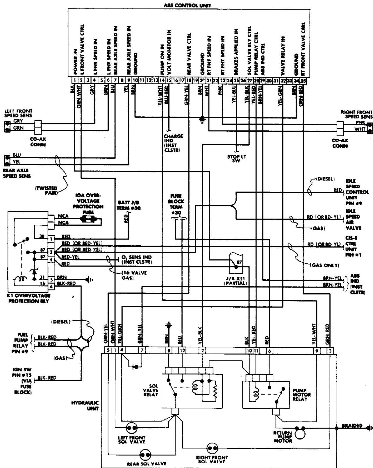
Fig. 4: Mercedes-Benz 190E Anti-Lock Brake System Wiring Diagram
