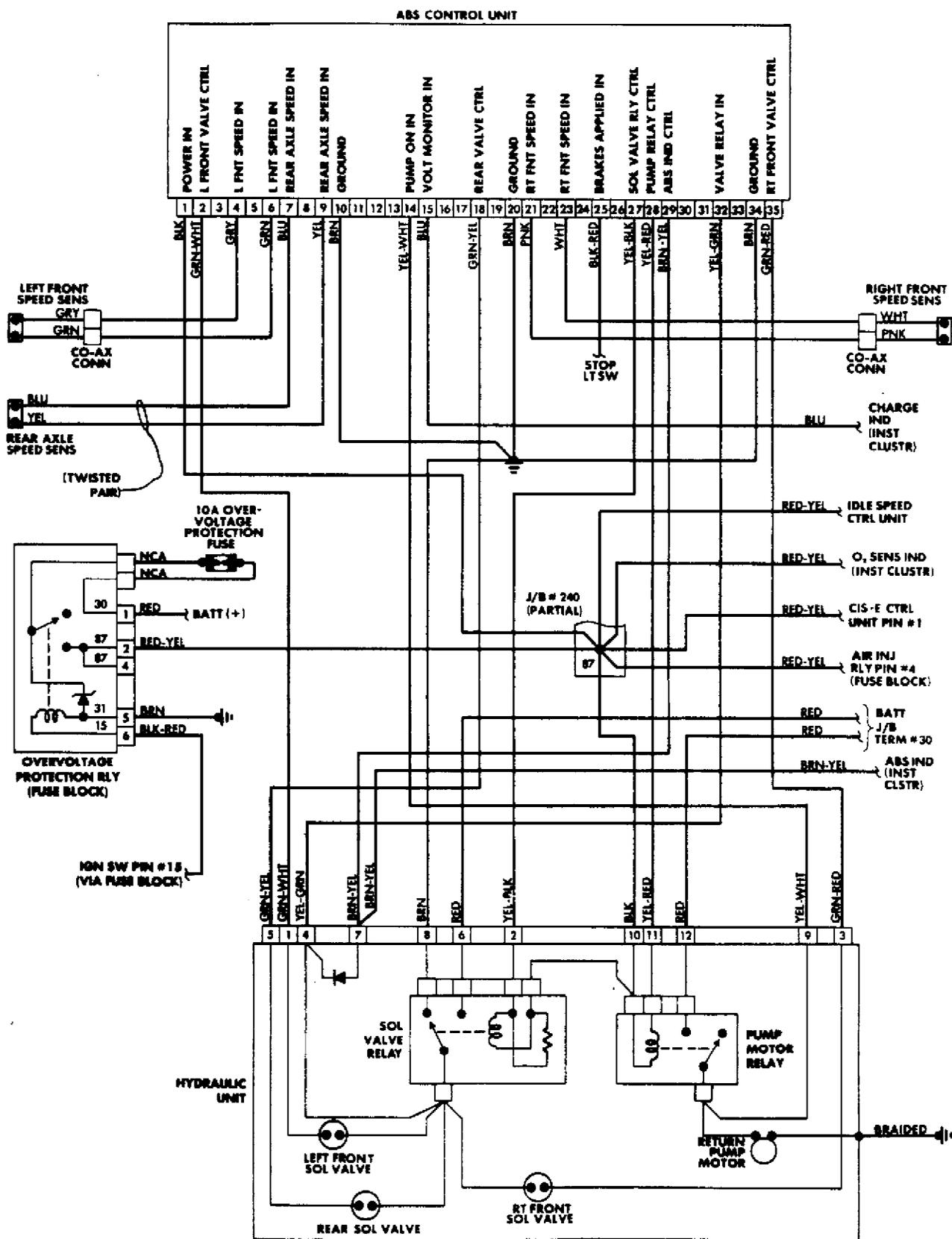
Fig. 7: Mercedes-Benz 560 Series Anti-Lock Brake System Wiring Diagram
