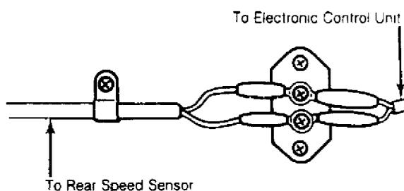
Fig. 3: Rear Speed Sensor Harness Connector (Under Rear Seat)
