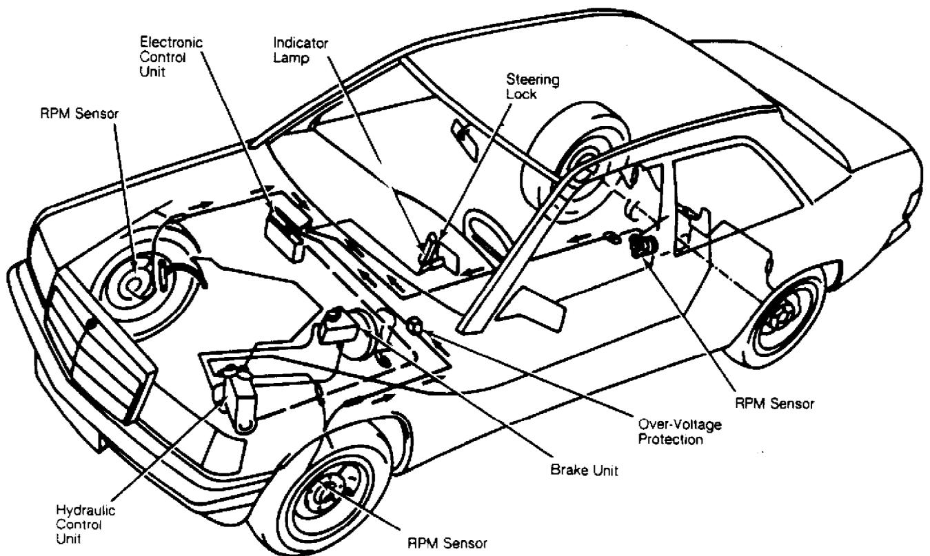
Fig. 1: Mercedes-Benz ABS Component Location
