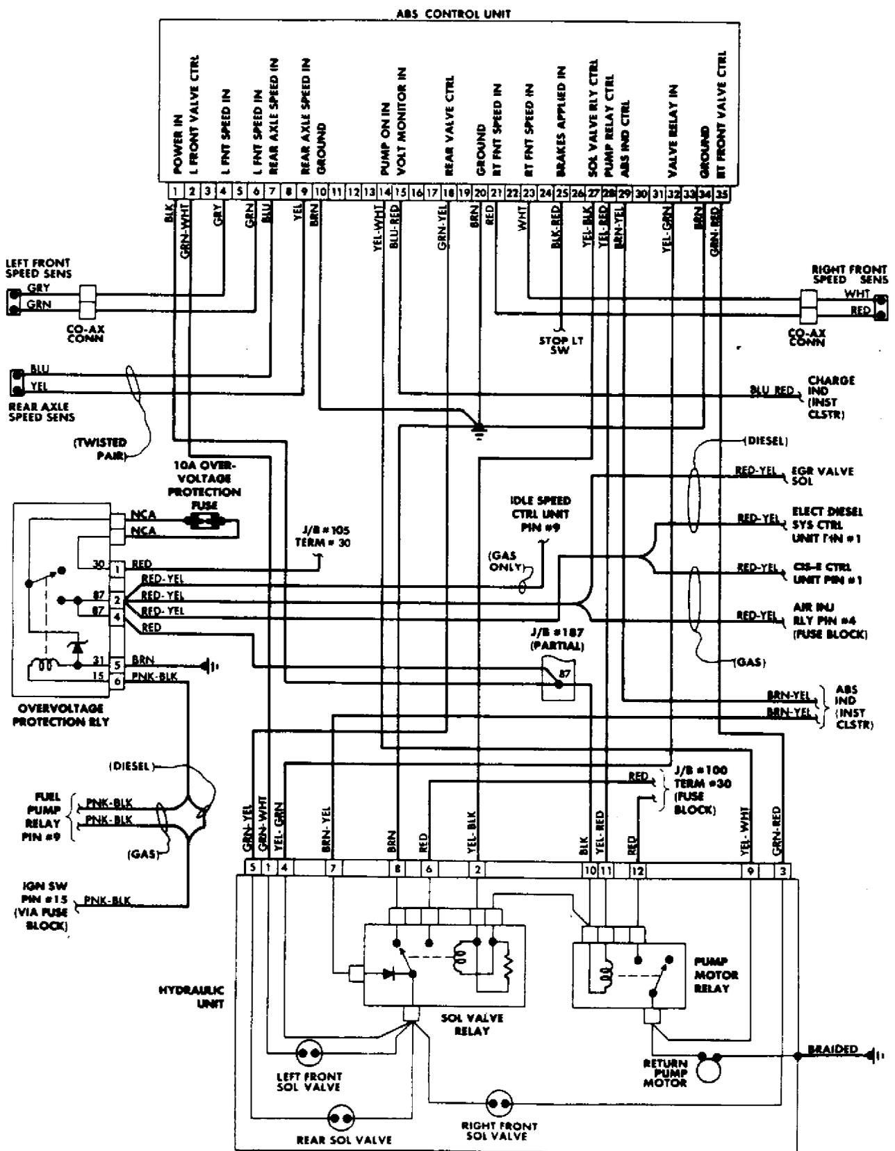
Fig. 6: Mercedes-Benz 420SEL Anti-Lock Brake System Wiring Diagram
