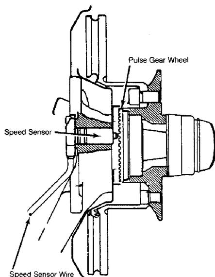
Fig. 2: Cutaway View Of Mercedes-Benz ABS Front Speed Sensor Assembly
