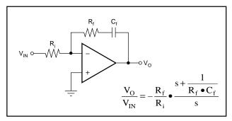
FIGURE 5. Integrator Circuit.
