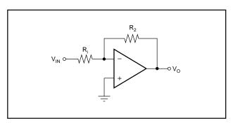
FIGURE 3. Inverting Gain Circuit.
