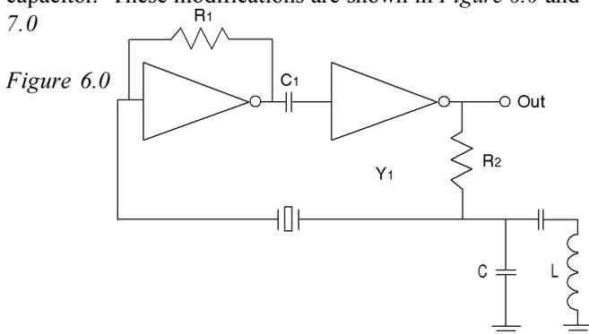
*Figure 6.0* depicts the modification of a series resonant circuit while *Figure 7.0* depicts the modification of a parallel resonant circuit.
