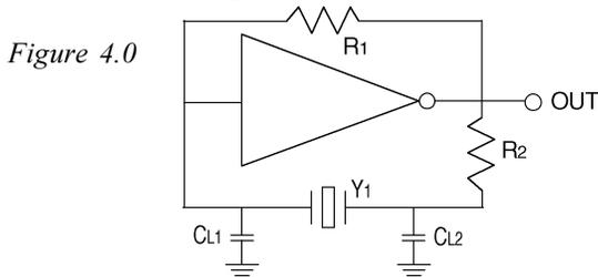
This circuit uses a single inverter, with two capacitors in the feedback loop. These capacitors comprise the “load capacitance” and together with the crystal unit, establish the frequency at which the oscillator will operate. As the value of the load capacitance is changed, so is the output frequency of the oscillator. Therefore, this circuit does provide a convenient means of adjusting the output frequency, should adjustment be required.
