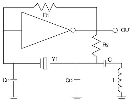
In both cases, the tank circuit is tuned to resonate at some frequency between the fundamental and the desired frequency. This results in the unwanted frequency being shunted to ground, leaving only the desired frequency being present at the output of the oscillator.
