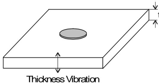
**Figure 15: Ceramic Element for Thickness Longitudinal Vibration**
