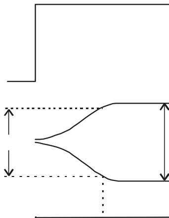
**Figure 20: Diagram of Oscillation Rise Time**
