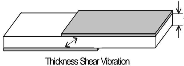
**Figure 14: Ceramic Element for Thickness Shear Vibration**
