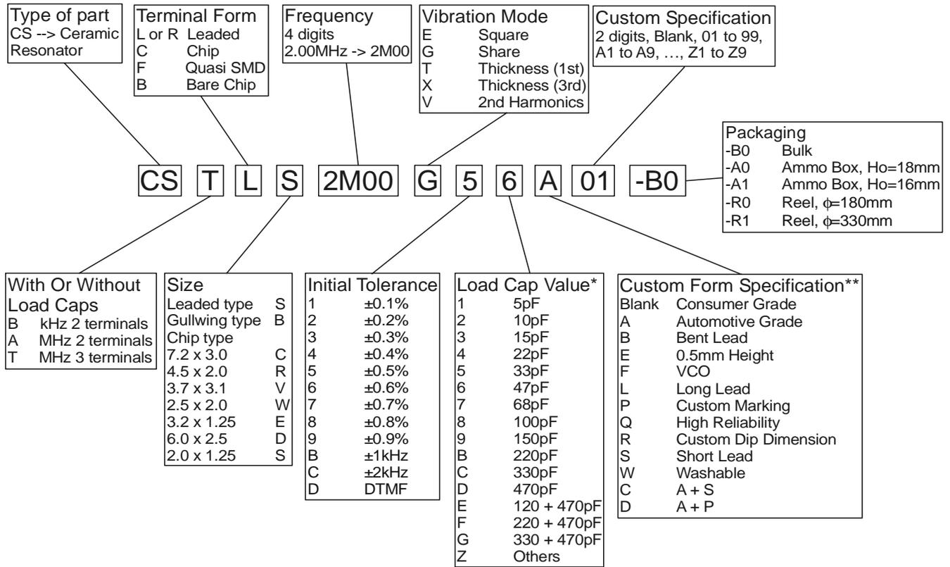
\* Note: Not all load cap values available with a specific part. In the case of 2 terminal resonators, cap value is for Murata standard circuit. In the case of 3 terminal resonators, cap value is for built-in capacitors.
