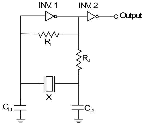
**Figure 19: Typical Hook-up Circuit for Ceramic Resonator**
