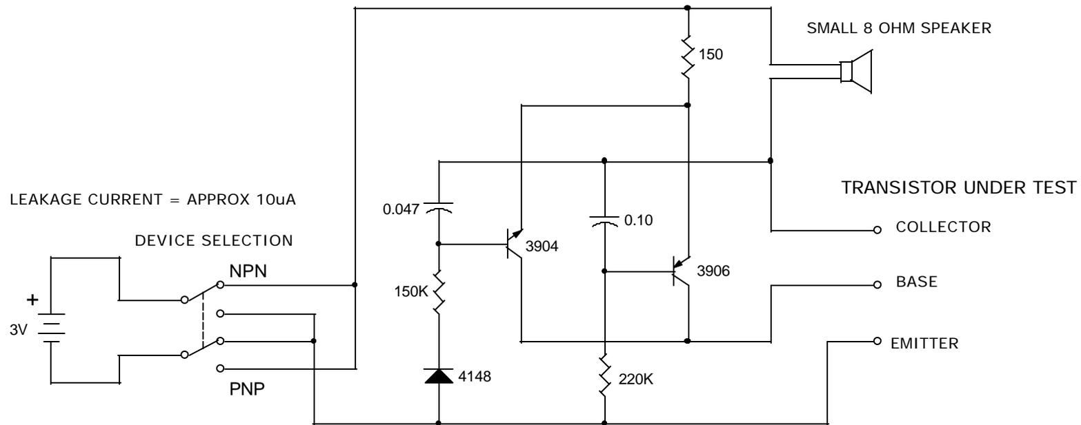
CIRCUIT IS AN OSCILLATOR THAT PRODUCES A TONE IN THE SPEAKER WHEN THE TRANSISTOR TESTS GOOD
