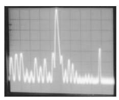
Figure 14—Output of a typical QRP transceiver kit. The 1-W plus output at 7 MHz is the dominant signal; all others are spurious outputs more than 40 dB down, currently meeting FCC specifications.
