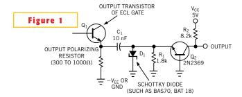
You don't need an expensive level-converter IC to provide a TTL-level trigger from an ECL-level signal.
