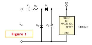
This SOT-23 IC with low-cost external components provides a combination of power-on reset and an efficient logic supply.
