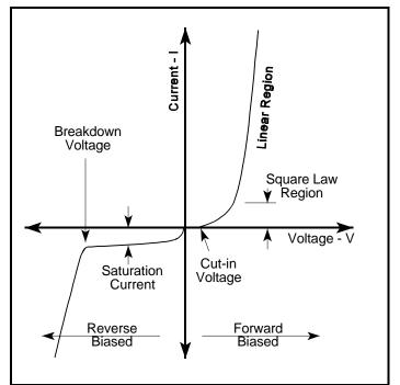
Figure 3. Diode Electrical Characteristics
