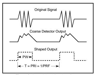
Figure 2. Demodulated Envelope Output
