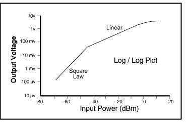
Figure 4. Diode Power/Voltage Characteristic
