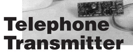
Receive telephone conversations on any FM radio with this neat little device.
