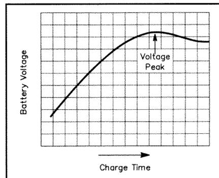
Figure 4—The terminal voltage of a NiCd cell increases as the cell is charged. Once the cell is fully charged, though, the terminal voltage drops slightly. Many of the so-called rapid or fast chargers detect this drop and automatically stop or reduce the charge rate. Two other techniques used to detect full charges in NiCds are time and temperature. Only NiCds that are specified as suitable for fast charging should be used in this type of charger.
