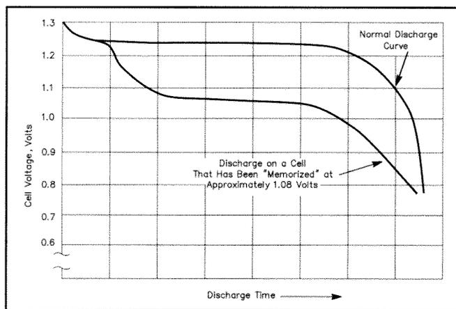
Figure 1—Discharge characteristics of a normal NiCd versus a cell with memory effect.
