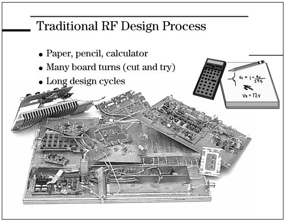
The traditional approach to RF design begins with a pad of paper, a pencil and a calculator (or slide rule for old-timers). Most of the critical aspects of the RF design are worked out with physical prototyping. The prototypes start out simple and then get more complicated as more circuits are added. At some point, the entire system is tested by connecting together the various circuits. This non-predictive process results in numerous board turns, which are time-consuming and expensive.
