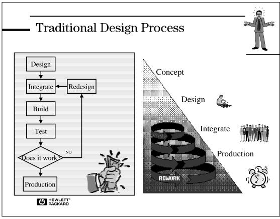
The problem is that this process is non-predictive. You hope that your design works, but in case it doesn't, you run multiple physical prototype boards varying some of the components hoping that one works. When it doesn't, you fall into "cut and try" mode, hoping each change you make fixes the problem, but you don't know that it will.
