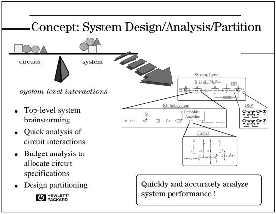
In the Modern Predictive Concept stage, EDA software facilitates exploring various system configurations. For each of the functional blocks in the system, individual behavioral models are used to analyze the overall system performance. Block and level budget analysis aids in design partitioning and circuit specification allocation. And as individual circuit design blocks are completed their effect on system performance is easily determined.
