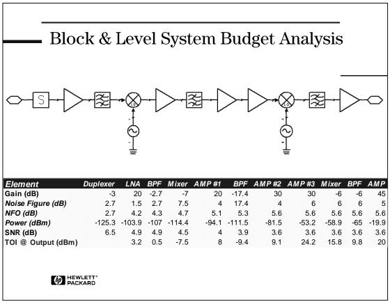
The system designer needs to make tradeoffs between the functional blocks of the design. Design partitioning and budget analysis are easily performed, allowing the analysis of all system-level parameters including gain, noise, and intermod measurements.
