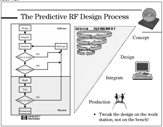
The key to success is the use of EDA software with accurate models early in the development process. The more design refinement that is performed in EDA software the fewer physical prototypes you'll need
