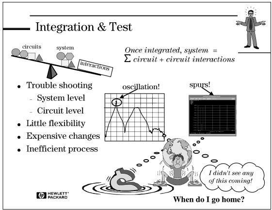
Once all the individual designs are completed, we integrate them to view the overall system performance. At this point, we typically notice that the system performance differs significantly from expected results. Even though all the individual circuits meet specifications when isolated, the circuit, when connected and overall system, does not.
