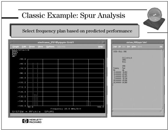
A classic example of a system-level design problem is spur analysis. Spurs from nonlinear devices such as mixers, diodes, and power amplifiers are another common problem for the system designer. In addition to predicting the frequency and level of spurs, spur analysis allows you to determine the best frequency plan (selection of IF frequencies) based on simulated results, making it easier to keep track of multiple spurs for complex subsystems, such as dual downconverters.
