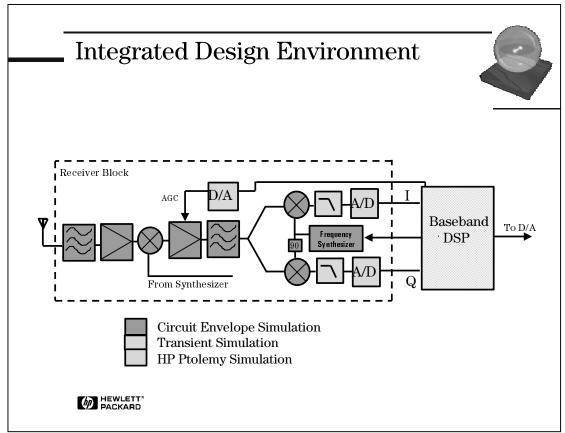
Today's mixed signal communications designs combine RF, analog, and digital circuitry. These individual designs are partitioned by the system-level designer early in the design process and are developed in isolation. It's only when they are integrated that the interactions between the DSP and RF circuitry are uncovered. Between 40% and 75% of the design effort at some companies is spent at the integration stage.
