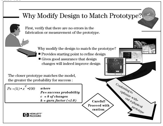
If the prototype performance differs from expectations, you need to do an initial check to verify that all the components, transmission line dimensions, connections, etc. are as specified. Once you are confident that the discrepancy does not lie in the fabrication of the prototype, the next step is to modify the design to match the behavior of the prototype.
