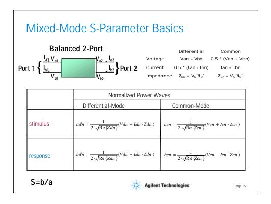
For a balanced device, we are not necessarily interested in voltages and currents referenced to ground. Instead, we can define differential and common mode voltages and currents on each balanced port. Likewise, we can also define differential-mode and common-mode impedances.
