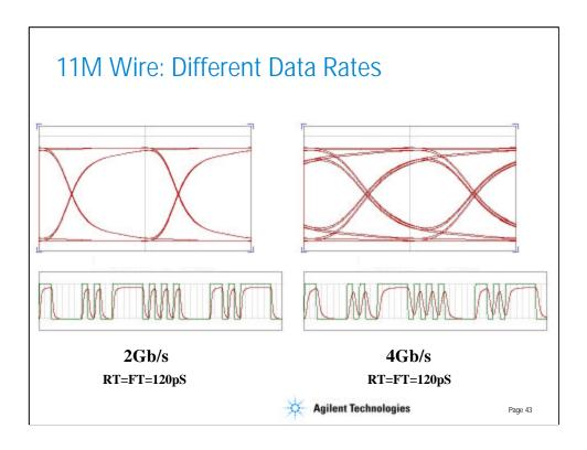
The graphs on the left show the result of using the differential mode sparameter data and generating an eye diagram. The driving function is a data rate of 2 Gb/s with rise and fall times of 120 pS, shown as the green trace below the eye. The resulting output waveform is overlaid in red, shifted in time to be synchronized with the input waveform. This output waveform is then used to generate the eye diagram above.
