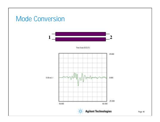
During the review of mixed-mode s-parameters in the frequency domain, we described the mode conversion parameters as being related to the asymmetry. In a perfectly symmetrical device, the mode conversion terms will be equal to zero. We can also examine the mode conversion parameters in the time domain. For example, the Scd21 of this transmission line are shown in this slide.
