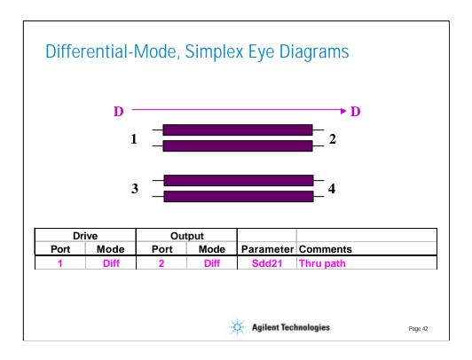
A Fibre Channel cable has two balanced pairs, one for sending data in each direction. The frequency domain measurements described here will fully describe the DUT provided the proper analysis is performed. So far we have concentrated on a single pair operating in one mode at a time. The next few slides will concentrate specifically on a single pair operating in differential mode.
