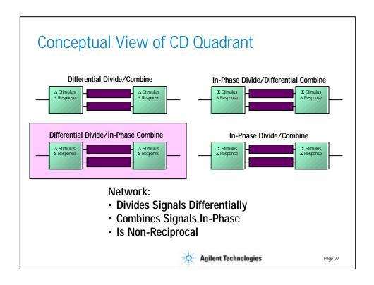
Once again we can convert the balanced port to a single-ended port to understand this mode more conceptually. In this case our network will have to divide the signal differentially as it propagates towards to DUT, and combine signals in-phase as they propagate away from the DUT. Therefore, our network will need to be non-reciprocal in addition to having perfect return loss, insertion loss, balance, and isolation.
