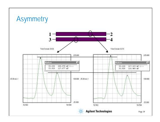
Like any physical device, this one is not perfectly symmetrical. This can be seen by comparing the path from 1-to-2 to that from 3-to-4. The responses look similar, but they are not exactly the same height, and they do not occur at exactly the same times. Therefore, how do we quantify the asymmetry of a balanced device with single-ended measurements?
