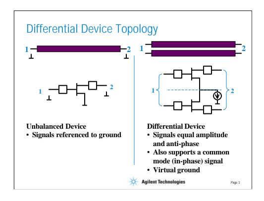
An unbalanced, or single-ended, device has all of its signals referenced to a common ground potential.
