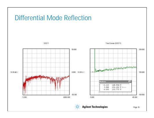
This data shows the differential input reflection performance in the frequency domain and the time domain. The time-domain data is the step response, formatted in ohms on the vertical axis. There is a large discontinuity on the input side as indicated by the spike. This may be responsible for the relatively poor return loss above 1.5GHz.
