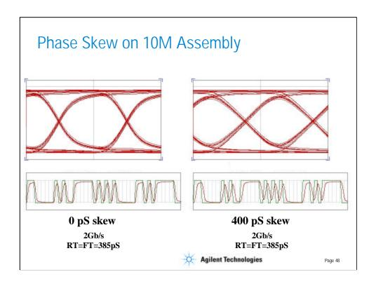
Of course the skew also has an effect on the eye diagram. On the left is the 10 M length of patch cord we have been examining. On the right is the same device with same driving function, but a skew of 400 pS has been introduced. As expected, the resulting eye has begun to collapse.
