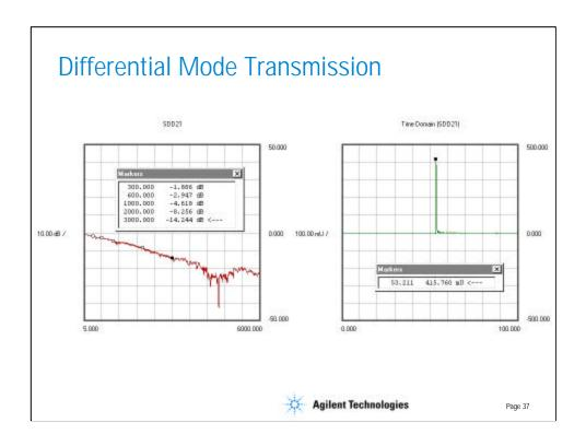
This data shows the differential forward transmission response in the frequency domain and the time domain. The time-domain data is the impulse response. The loss with frequency increases approximately linearly up to about 3 GHz. The group delay is about 53.2 nS.
