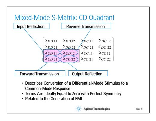
The parameters in the lower left corner describe the common-mode response of a device to a differential stimulus. As with the other modes, there are reflection parameters on each port, and transmission parameters in each direction.
