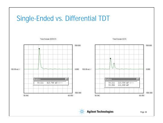
Often engineers will try to characterize the between-pair skew by making two single-ended measurements, one on each side of the pair. This can lead to misleading conclusions.
