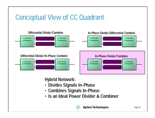
The balanced ports can also be converted to single-ended ports with an ideal power divider/combiner. In this case, the performance will be isolated to the common mode. The s-parameters of the resulting 2-port single-ended network are the s-parameters in the CC quadrant of the mixed-mode s-matrix.
