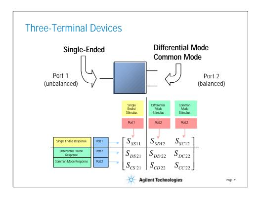
The balanced device that was examined until now has had two balanced ports. A simple extension of the mixed-mode concept can be applied to devices having a combination of balanced and single-ended ports. In this scenario, we need to consider differential and common modes on the balanced ports, and one mode on the single-ended port.
