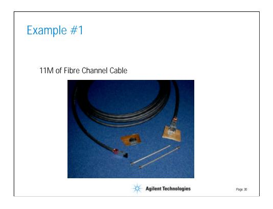
The first device to be considered will be an 11M length of cable. The interface is through SMA connectors attached to short lengths of semi-rigid cable. These semi-rigid cables were characterized to allow them to be de-embedded later.
