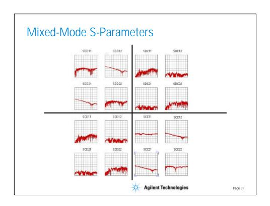
The mixed-mode s-parameters of this cable are shown on this slide. The parameters upper left quadrant describe the behavior in the differential mode. They show a return loss of 20dB at the low end of the band, increasing to about 8dB at the worst point. The loss increases linearly to about 15dB.
