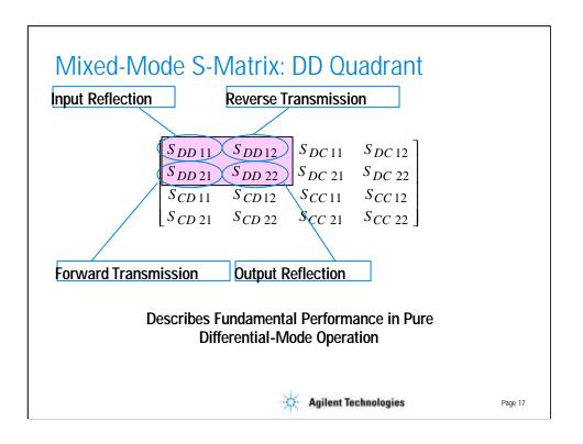
For a device with two balanced ports, the quadrant in the upper left corner of the mixed-mode s-matrix describes the performance with a differential stimulus and differential response. When the performance of the device is isolated to this specific mode, these four parameters describe the input and output reflections, and the forward and reverse transmissions much in the same way a 2-port s-matrix describes the performance of a single-ended device.
