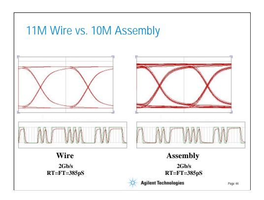
This graph compares a length of cable with de-embedded SMA connectors with a patch cable consisting of approximately the same length of cable plus two high speed connectors. Comparing these diagrams clearly shows a degradation in the eye diagram resulting from the electrical performance of the connectors.
