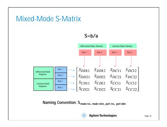
Again we can take a ratio of all of the possible combinations of response over stimulus for the differential and common-mode normalized power waves to calculate the mixed-mode s-parameters.
