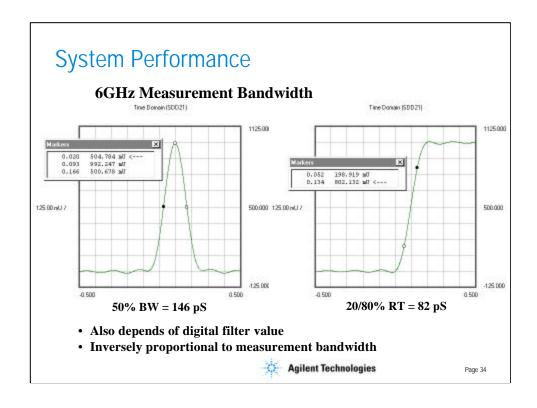
These graphs show the TDT response of the 6GHz system with a through connection (no DUT). This shows the effective impulse width and step rise time. These times are proportional to the maximum measurement frequency, so the pulse width of the 20GHz system is 44pS, and the rise time is 25pS.
