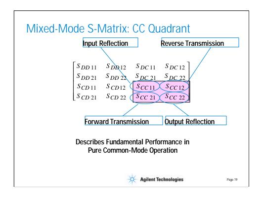
For a device with two balanced ports, the quadrant in the lower right corner of the mixed-mode s-matrix describes the performance with a common-mode stimulus and a common-mode response. When the performance of the device is isolated to this specific mode, these four parameters describe the input and output reflections, and the forward and reverse transmissions.
