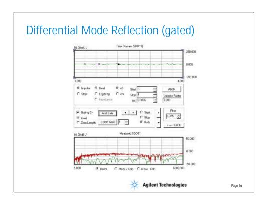
We may want to know what effect the large discontinuity at the input has on the frequency-domain response. The graph at the top of this page shows the time domain response of this device, but with the discontinuity "gated," or mathematically removed.
