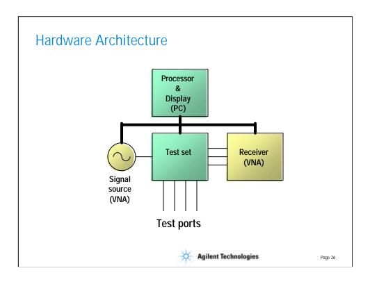
The system that measures balanced devices and display mixed-mode sparameters, uses a combination of hardware and software from Agilent. A 6 GHz system is available using the 8753 VNA and E8357A PNA, as is a 20 GHz system using the 8720.
