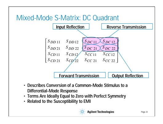
Finally, the parameters in the upper right corner describe the differential response of a device to a common-mode stimulus. Again, there are reflection parameters on each port, and transmission parameters in each direction.
