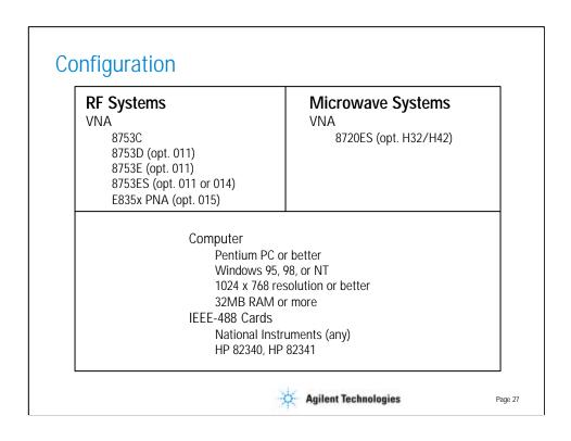
The 6 GHz system that works with the 8753 uses a test set. The 8753 VNA requires either the delete test set option (011) or the configurable test set option (014).
