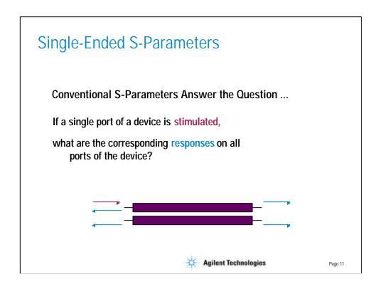
Let's compare what is meant by single-ended and mixed-mode s-parameters. Recall that with conventional single-ended s-parameters we are describing the performance of a device when it is stimulated on a single port, and the corresponding responses are observed on all of the ports.
