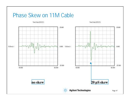
As described earlier, the mode-conversion terms can be used to help determine the cause of asymmetry in a DUT. Even a slight asymmetry can be observed in the time domain. For example, the graph on the left shows the Scd21 parameter of the 11M Fibre Channel cable. If a phase skew of only 20 pS is introduced, the result can be clearly observed, as shown in the graph on the right.
