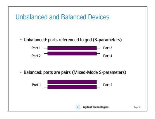
A multi-terminal device can be viewed in different ways, depending on how it is meant to be operated. For a device that is designed to be a single-ended four-port, its conventional four-port s-parameters can be measured and displayed.
