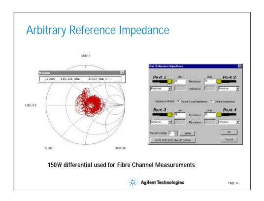
The reference impedance has been set to  $150\Omega$  differential for this device. When a marker is placed at the Sdd11 display at the low end of the band, the impedance readout of the marker confirms that the impedance of the cable is nominally  $150\Omega$ .
