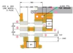
RESISTOR R1: 150 Ohm, 0805 SIZE CAPACITOR C1: 1.5 pF, 0805 SIZE RECOMMENDED MATERIAL: ROGERS R04350, DIELECTRIC THICKMESS: .030 ± .002 COPPER: 1 0Z. EACH SIDE
