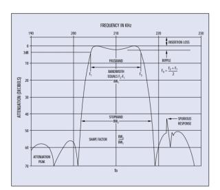
Insertion Loss — Power loss of the filter in the passband (in dB). Zero dB reference shall be the point of maximum output of the filter unless it is specified otherwise.
